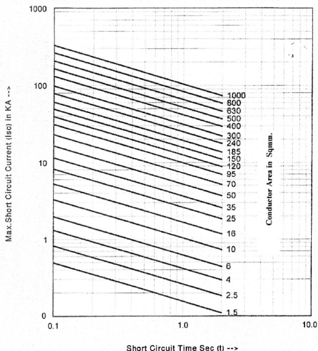
Short Circuit Curves For Copper Conductor
